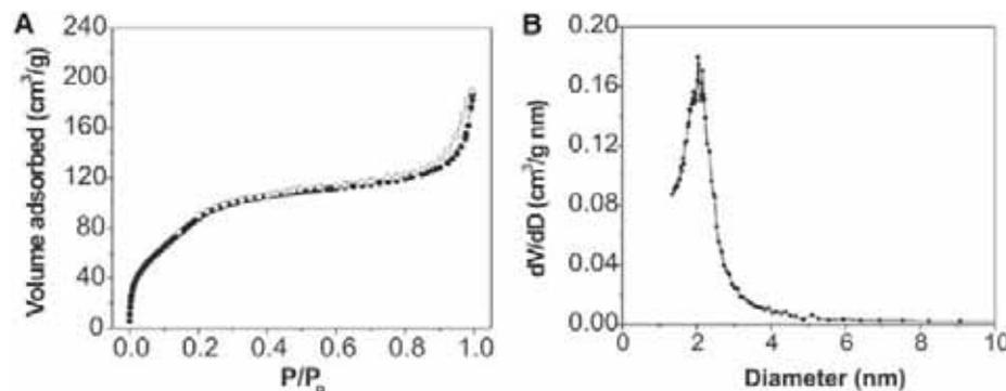
**Fig. 3.** (A) Nitrogen adsorption-desorption isotherms at 77 K of heat-treated  $\text{NH}_4^+$ -exchanged MSU-Ge-2 (solid circles, adsorption data; open circles, desorption data). The hysteresis observed at  $P/P_0 > 0.8$  is due to the interparticle voids between the agglomerated particles. (B) BJH pore size distribution calculated from the adsorption branch of the isotherm.
