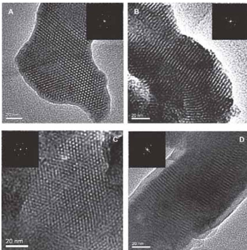
**Fig. 2.** TEM and (insets) FFT images. (A and B) As-prepared MSU-Ge-2. (C and D) Mesoporous MSU-Ge-2 obtained by heat-treating the  $\text{NH}_4^+$ -exchanged material. The images show a periodic hexagonal array along the [100] direction (A and C) and a periodic array of parallel pore channels along the [110] direction (B and D).
