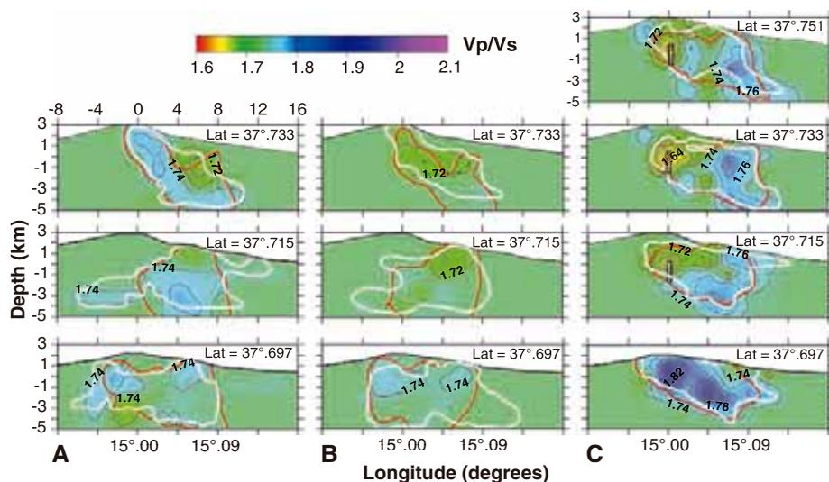
**Fig. 4.** W-E cross sections showing the variation of the  $V_p/V_s$  ratio during the pre-eruptive periods [(A) and (B)] and the 2002–2003 eruption (C). The vertical black rectangle in (C) indicates the location of the 2002–2003 dike intrusion, as modeled by geodetic data in the southern flank (19, 20). The white and red lines indicate the well-resolved regions of the model with SF values  $<2$  and derivative weight sum values  $>50$ , respectively (SOM text).
