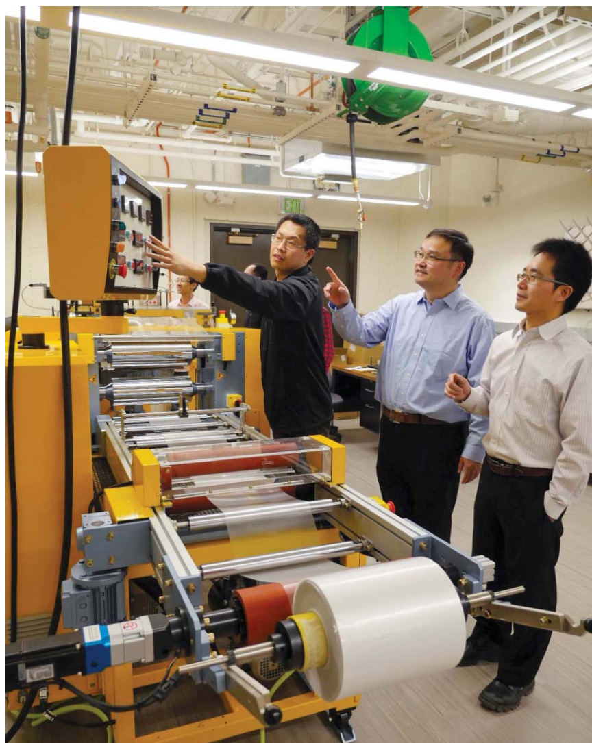
FIGURE 1. YAOGUANG MA, XIAOBO YIN, AND RONGGUI YANG (left to right) oversee the roll-to-roll production of the glass-polymer film used in their radiative cooling experiments.
