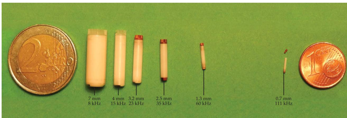
**FIGURE 1. IN MAGIC-ANGLE SPINNING NMR**, a sample is loaded into a cylindrical rotor that is spun rapidly to mimic the effects of molecules tumbling in a fluid. As shown here, the maximum spinning frequency depends on the rotor diameter. The smallest rotor, 0.7 mm in diameter, was recently debuted. (Courtesy of Guido Pintacuda.)
