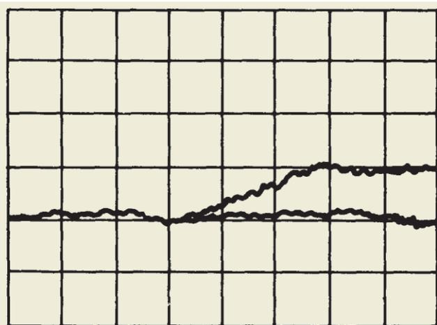
**FIGURE 2. PROOF OF CONCEPT.** This oscilloscope trace—gridline spacings are 1 mV (vertical) and 0.4 ns (horizontal)—from Juri Matisoo’s 1966 paper demonstrated that Josephson junctions could switch from a supercurrent, pair-tunneling state (0 V signal) to a dissipative, single-particle-tunneling state (1 mV signal) in less than 1 ns. (From J. Matisoo, *Appl. Phys. Lett.* **9**, 167, 1966.)
