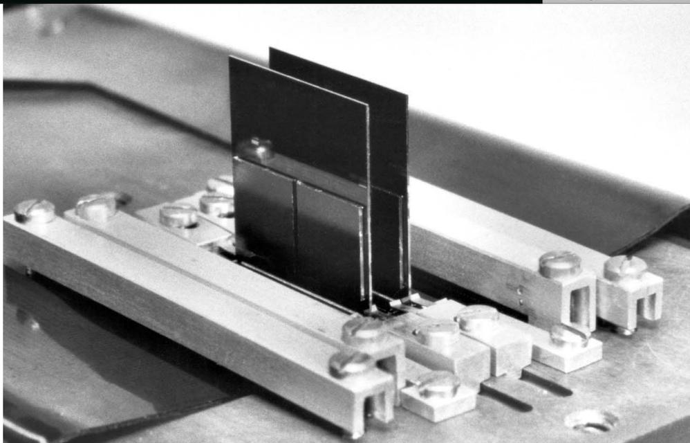
**FIGURE 3. PROTOTYPE CHIPS.** In the early 1980s, IBM fabricated experimental Josephson chips to test their performance and identify potential manufacturing problems. This photograph shows a chip assembly containing two cards (large squares). Two 6.4 mm × 6.4 mm Josephson chips (small squares), are attached to each card. (Courtesy of IBM.)
