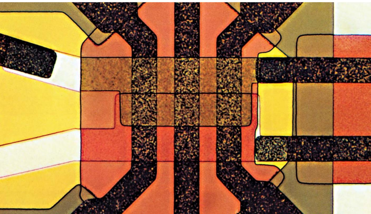
**FIGURE 1. IBM JOSEPHSON CIRCUIT** from 1974. Josephson junctions are formed at the intersection of perpendicular superconducting strips (dark areas) with an insulating oxide layer sandwiched between the two. (Courtesy of IBM.)
