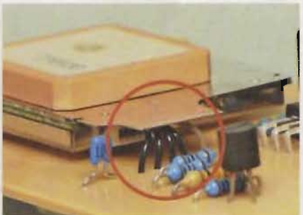
This close-up view shows how the EM-408 is connected to the PC board via the 5-way interface cable supplied with the module – see text.
