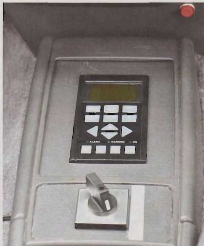
The large knob in the foreground is the Forward/Neutral/Reverse switch, with the Danfoss keypad and display. It is not possible to inadvertently throw the car into reverse while under way. This is prevented by a key interlock which must be used to change motor direction.
