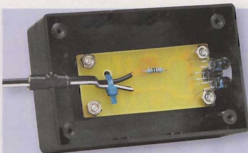
The IR Source board carries the three infrared LEDs (LEDs1-3) plus an 820Ω current-limiting resistor. It's mounted inside a UB5 case on 6mm untapped spacers and derives its power from the Detector unit.
