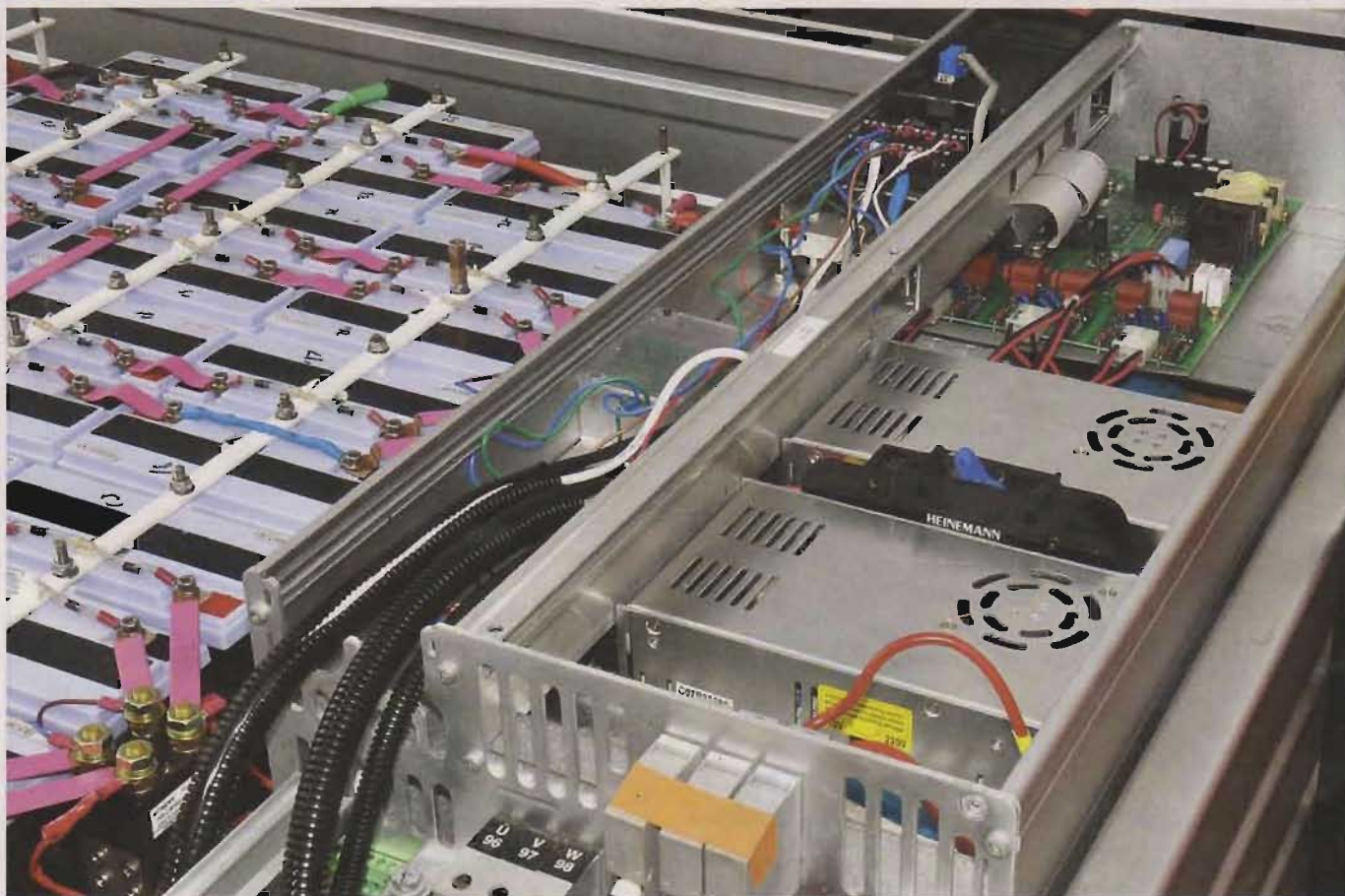
This shot show the Danfoss VLT5024 frequency converter with the top cover removed. In the foreground you can see the two 13.8V 25A switchmode power supplies which are used to charge the 12V ancillary battery. They occupy the space originally taken up by the 415V 3-phase rectifier filters.
