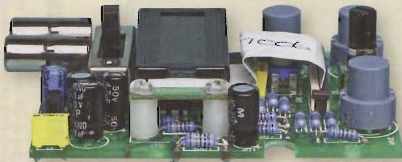
This side-on view shows how the LCD module is secured to the PC board using Nylon spacers and screws.
