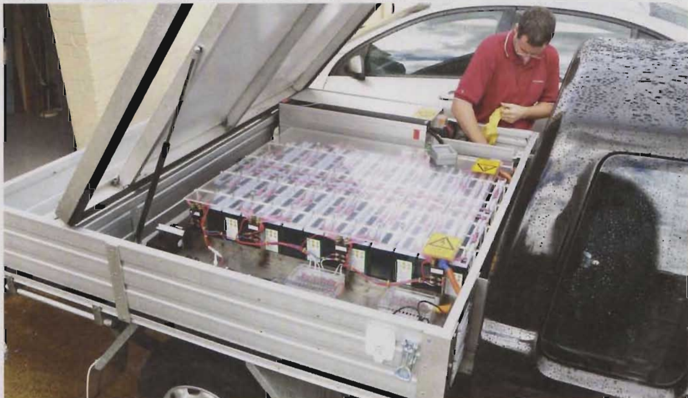
Mal Faed drying off the electronics while we took photos of his EV conversion on a (very!) wet day. This is looking across the battery bank with the Danfoss VLT5042 controller under his right elbow.
