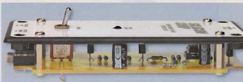
Above: the Detector board is secured to the lid of the UB3 case using four M3 x 15mm tapped spacers and eight M3 x 6mm machine screws
