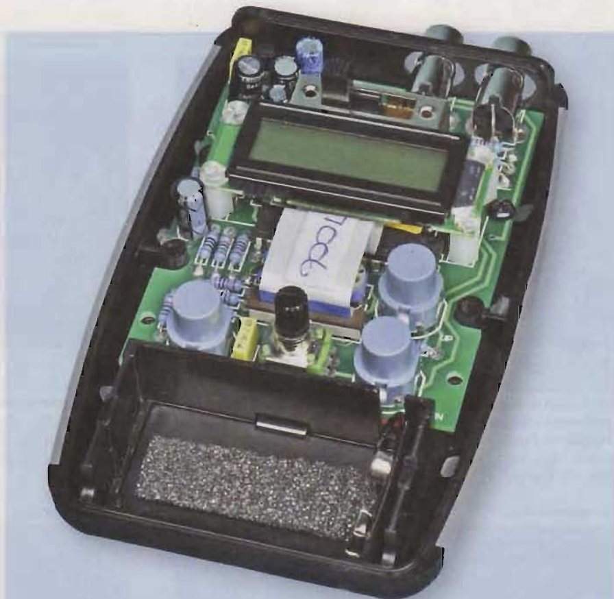
The PC board is secured inside the case using metal screws that go into integral mounting posts. Note that the battery leads are run under the PC board and into the battery compartment via a slot in the back wall.
