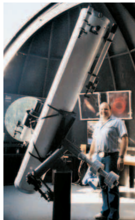
MacDonald with his custom-built 12½-inch f/7.5 Newtonian reflector and 5-inch f/8 refractor. He has plans to replace the instrument with a telescope in the 20- to 25-inch range.
