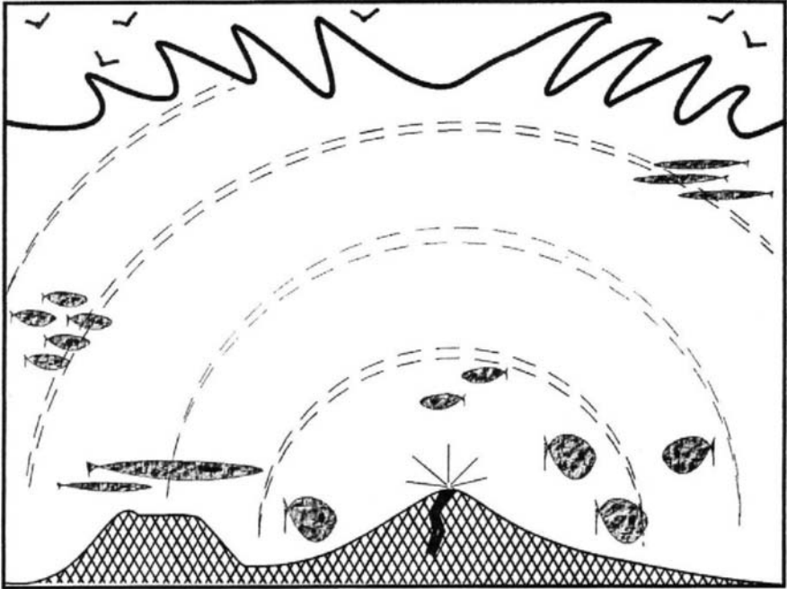
Figure 1.5: Schematic showing the formation of tidal (transverse) surface waves from a deep disturbance propagated to the surface by longitudinal waves.
