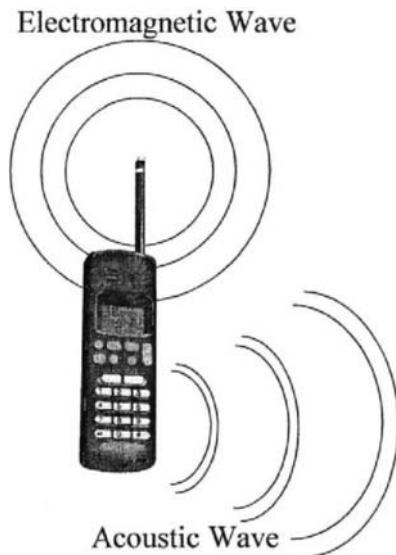
Figure 1.1: Acoustic and electromagnetic waves from a cell phone.
