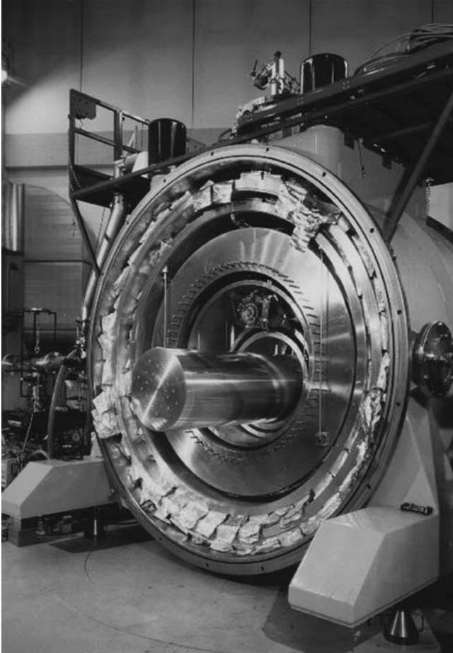
FIGURE 6.3 The AURIGA resonant bar, located at the Legnaro INFN labs, is enclosed within a large multi-layer container. In this photo the container is open, to give a full view of the cylinder located at the center. The role of the container is to provide the bar with thermal and seismic isolation. (Picture courtesy of the AURIGA collaboration)
