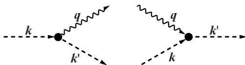
Fig. 13.4. Two types of Raman scattering. In Stokes processes a phonon is emitted; in anti-Stokes processes a phonon is absorbed
