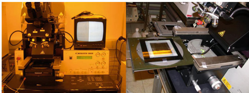
Fig. 4.18 Photolithography instrument for anode patterning
